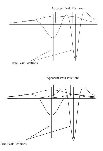
Figure 207: Apparent and True Peak Position
