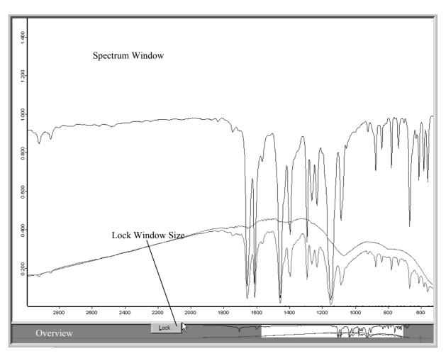
Figure 14: Spectrum and overview window showing lock button
