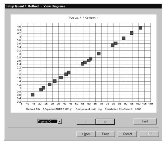
Figure 191: Graphic Display of Calibration Results – True vs X
