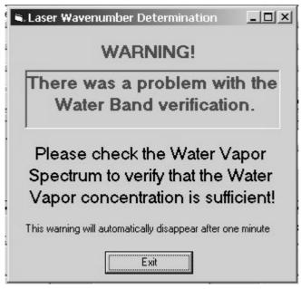
Figure 294: OVP - Water vapor warning
