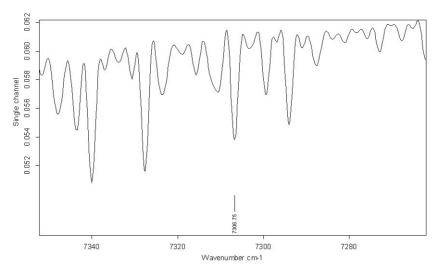
Figure 335: NIR water vapor spectrum
