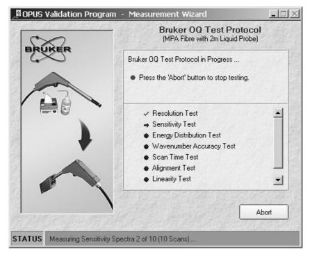
Figure 306: OVP - Measurement Wizard with OQ Test Protocol
