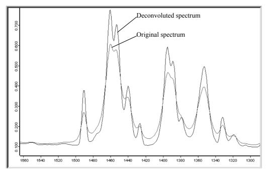
Figure 144: Spectrum before and after Fourier Self-Deconvolution
