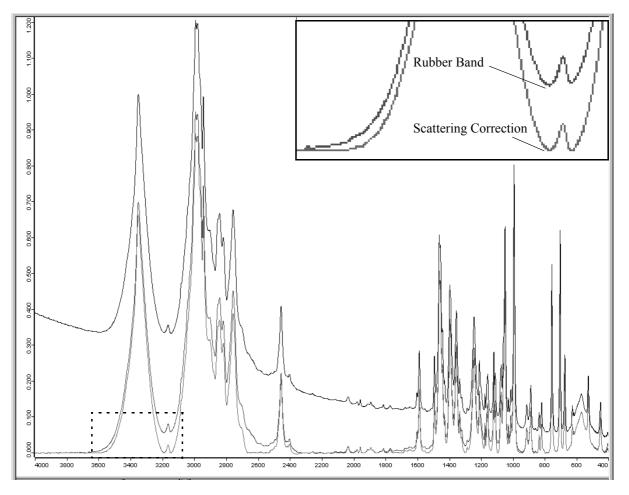
Figure 108: Spectrum prior to and after Baseline Correction
