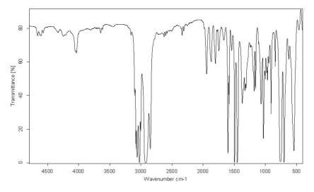
Figure 336: Polystyrene spectrum for MIR
