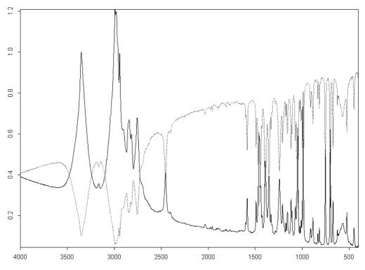
Figure 115: Converted Absorbance Spectrum into a Transmittance Spectrum
