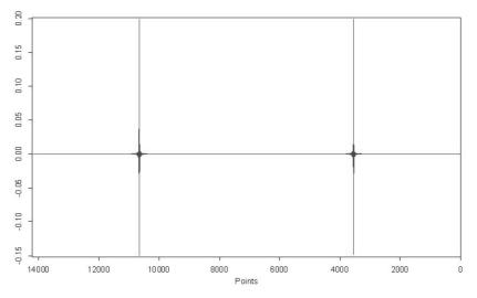
Figure 318: Double-sided interferogram
