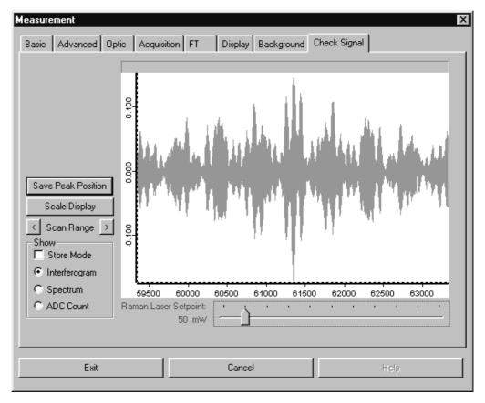
The laser power can be set using the slider on the *Check Signal* tab. The actual performance will be displayed.
