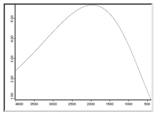
Figure 133: Radiation emitted by a black body at 1000K
