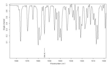
Figure 321: MIR water vapor spectrum
