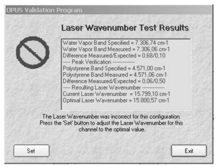
Figure 295: OVP - Laser Wave Number Test Results
