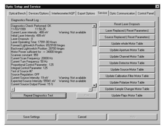
Figure 71: Optic Setup and Service - Service tab
