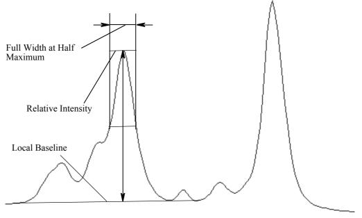
Figure 204: Spectrum with Line width, Relative Intensity and Baseline Indicated
