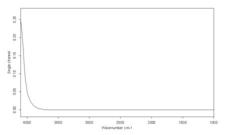
Figure 339: Single-channel spectrum around detector cutoff frequency
