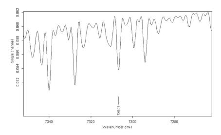
Figure 322: NIR water vapor spectrum
