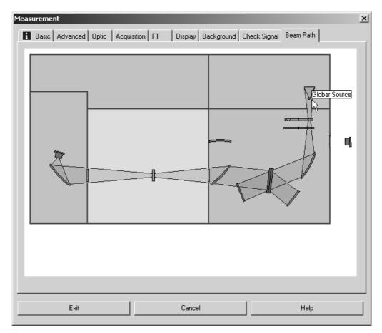
Figure 92: Measurement - Beam Path tab (Tensor 27)
