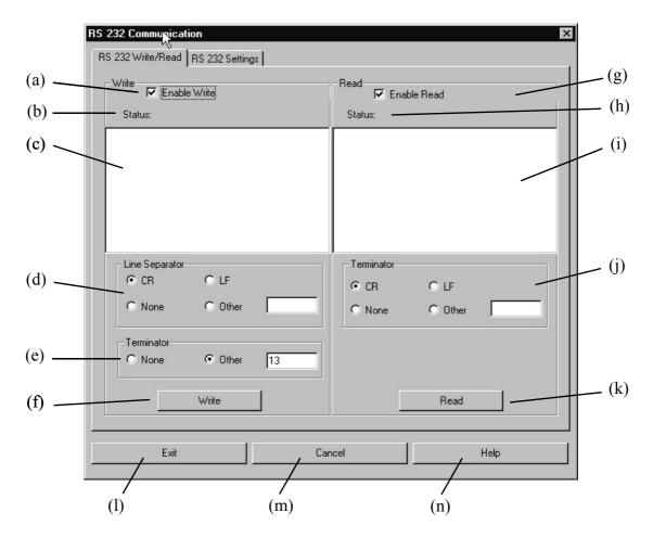
Figure 36: RS 232 Communication - RS 232 Write/Read tab
