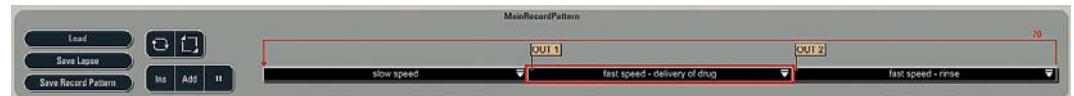
Fig 10: The Record Pattern. A 20x looping has been defined for the whole experiment. In Job2 and Job 3 a trigger out has been set up.
