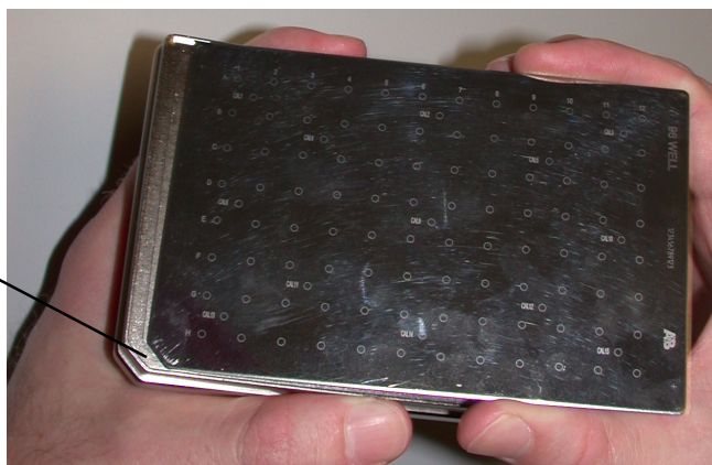
Figure 3-5 Assembling an Opti-TOF™ Plate
