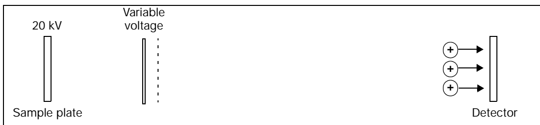
Figure 1-5 Time-delay extraction enables velocity focusing
